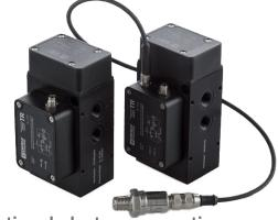
Extremely fast (2.5ms) and very accurate (+/-0.1%), TR proportional electro pneumatic pressure regulators convert a voltage or current input into a precise proportional pressure output. Direct-acting voice-coil technology inside these valves removes minimum pressure requirements and delivers smooth, accurate air pressure control down to 0 psig and below.
